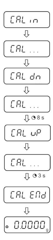
In case of the adjustment error (e.g. object on the plate) the following error message will be displayed: <CAL NO>, repeat the adjustment procedure.
